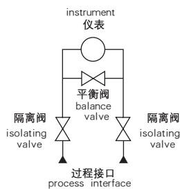
特殊出口位置的三阀组3-valve manifold on special outlet position.
